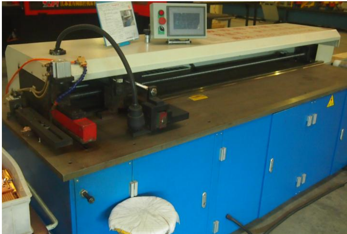
Used for cutting large quantities of fixed dimension length of CCA busbar
