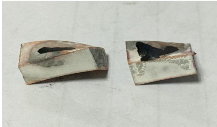
Fig.15 Penetration test of the longitudinal section
