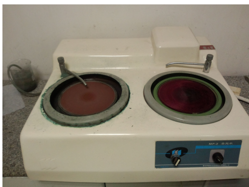
Fig.6 MP-2 polishing machine
