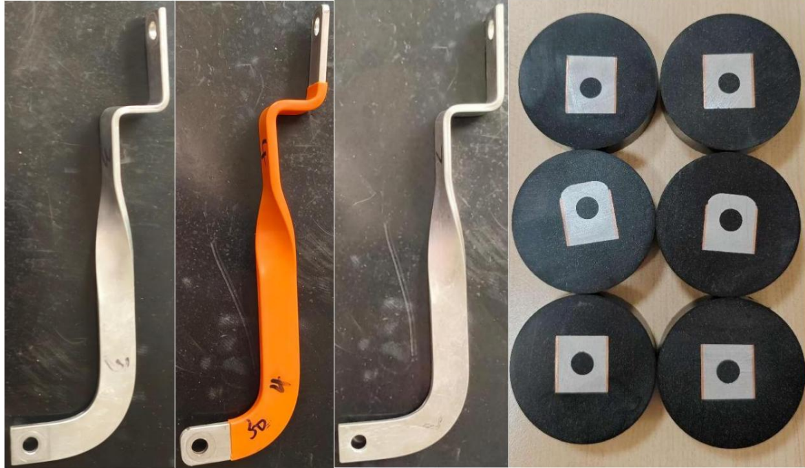
3.1 Among them, No. 3 and No. 8 are tin-plated products with full coating. The surface coating is visible and not corroded, and the substrate is protected and not corroded.
