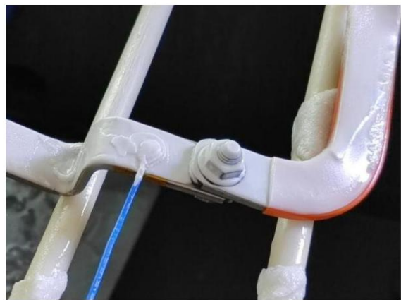
A partial photograph taken after 500 hours of salt spray (1 mm of salt deposited on the upper surface).
